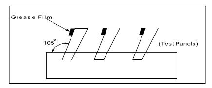
After 18 hours of 400°F continuous heat in a static position, the surface of the LUBRIPLATE High Temp was dark brown, but the lubricant was soft and greasy and under the surface had not changed color.
